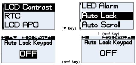
Select the Auto Lock by press ▼ key to select "Auto Lock" then press ← key to review. Press ■ key to accept or press ← key then press ▼ key to change and press ← key to confirm.
