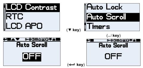
Select the Autoscroll by press ▼ key to select "Auto Scroll" then press ← key to review. Press ■ key to accept or press ← key then press ▼ key to change and press ← key to confirm.
