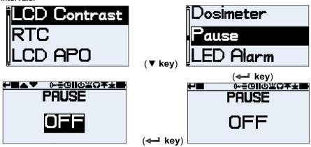
Select the Pause function by press ▼ key to select "Pause" then press ← key to review. Press ■ key to accept or press ← key then press ▼ key to change and press ← key to confirm.
