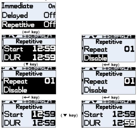
In the Timers mode, press ▼ key to select "**Repetitive**" then press ← key to review the Start-time and Duration-time, press ▼ key to review the Repeat times. If you will change the data, using ← key to position the cursor to the time element to adjust then using ♠, ▼ keys to setting the selected time element value including the Repeat number from 01 to 99 and the "**Enable**" or "**Disable**" selected. Press ← key to confirm then press ► key to exit.
