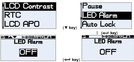
Select the LED alarm by press ▼ key to select "**LED Alarm**" then press ← key to review. Press ■ key to accept or press ← key then press ▼ key to change and press ← key to confirm.
