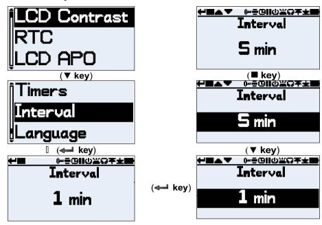
The LAVG, LEQ, LCPK and LZPK time-history data is saved at an data memory interval time for every run and are available following download. Data memory interval time can be set by press ▼ key to select "Interval" then press ◆ key to review. Press ■ key to accept or press ◆ key then press ▼ key to select 1, 5, 10 or 30 minute, 1 or 2 hours and press ■ key to confirm.
