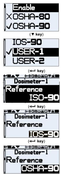
In the pre-difined setup mode, press ▲, ▼ keys to select the desired customized configuration from "USER-1" to "USER-9" then press ← key to confirm. Press ▲, ▼ keys to review the parameters, if you will change the parameters press ← key to confirm then press ▲, ▼ keys to change the desired parameters value and press ← key again to save.
