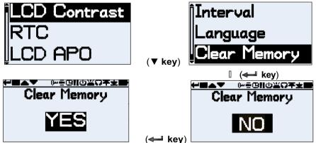
In the setting mode, press ▼ key to select "Clear Memory" then press ← key to enter this mode. Press ▼ key to select "YES" then press ← key to the additional screen "Clear Memory A Sure?" is displayed to check that you wish to progress since once cleared all stored runs will be lost.
