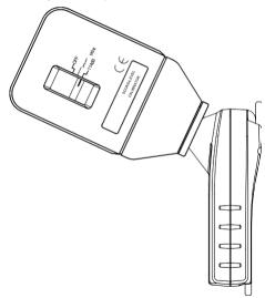
The meter will automatically recognize a 1kHz calibration tone and enter the calibration mode.
